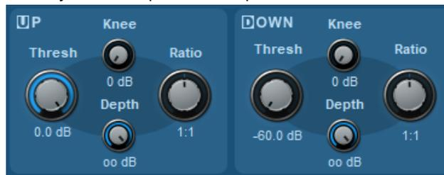
The **up threshold** and **down threshold** correspond to the upper part and lower part of the dynamics response curve. They let you specify the upper part (usually for compression) and lower part (usually for gating) of the curve independently:
