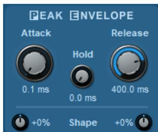
Use attack and release shape to fine tune the time response
