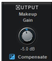
To simplify this task, you can use the compensate (auto-gain) feature that normalizes the response curve (0dB input produces 0dB output). The make-up gain is then applied after the normalization occurs. So beware that activating/ deactivating the auto gain feature when make-up is used might result in a very large volume increase. Be sure to use the output limiter to avoid damaging your speakers or your ears.
