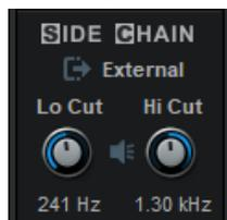
The side chain filter is used to choose which frequencies in the audio content trigger the effect. It is applied to the selected side chain signal (either after the input filter for internal side chain, or to the external side chain signal). It is not directly audible because it processes the side chain signal, only used to trigger the volume control.
