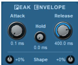
If all these parameters are set to 0, you obtain a wave shaper/ distortion unit. We advise you to add a low- pass filter after the unit if you wish to keep a pleasant sound, and use at least 2x oversampling (1 stage) to avoid aliasing.
