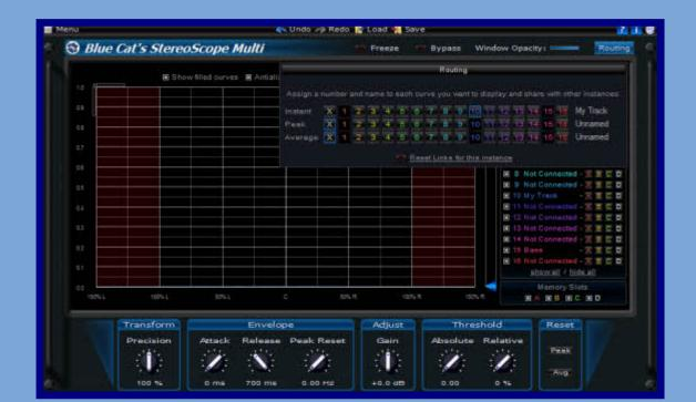
The stereo scopes show exactly how a signal is spread across the stereo field. This is an amazing aid in keeping sounds and mixes balanced. Another key use for the Stereo Scopes is for uncovering phase issues. A lot of effects can cause phase problems. With the scopes, you are able to see how each effect is affecting the stereo field. This allows you to deal with phase issues at the root of the problem. ⋛
