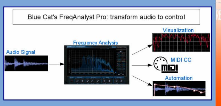
They also have a routing buss that you can go into and click on the curves 1 through 16. Now you can view all signals at once from one of the four instances. The routing bus offers four different ways to analyse the audio. Even more outstanding is the fact that each of the 16 curves can be named so that on the analysis view you know exactly which is
